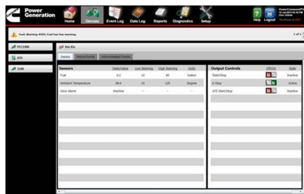
Clicking on the Home Page building icon navigates the user to the details page, providing a snapshot of all configured sensors or output controls.
